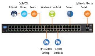
Typical Network Configuration for the SLM2048
