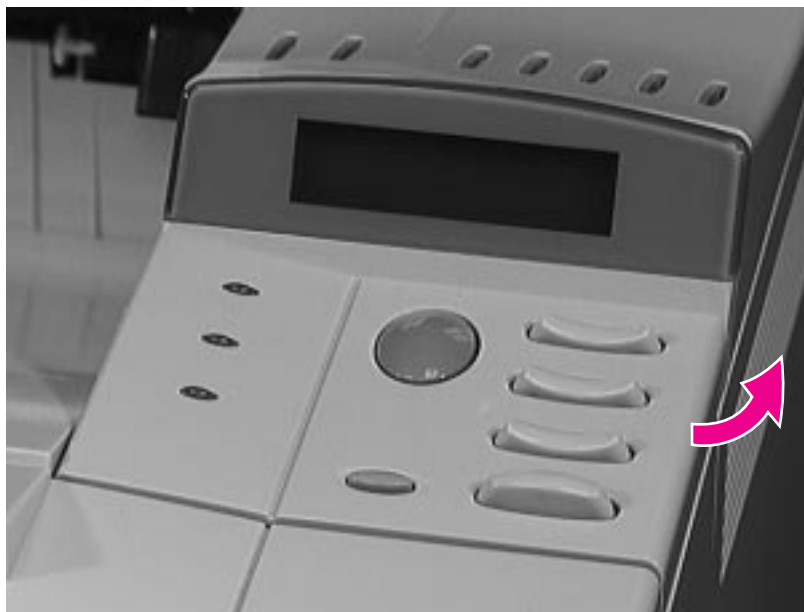
Figure 6-3 Removing the Control Panel Overlay
