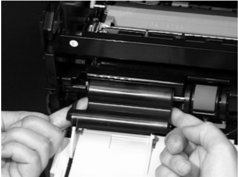
Figure 6-12 Removing the Tray 1 Sensor Arm Cover
