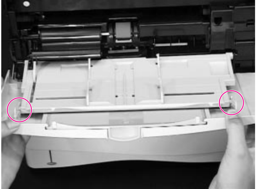
Figure 6-11 Removing Tray 1 from the Front Cover
