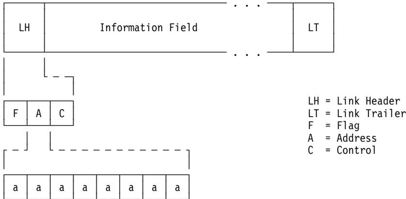
Figure 1-3. Address Field of Link Header. (aaaaaaaa)
