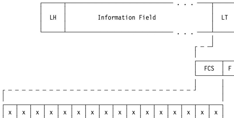
Figure 1-8. Frame Check Sequence Field of Link Trailer
