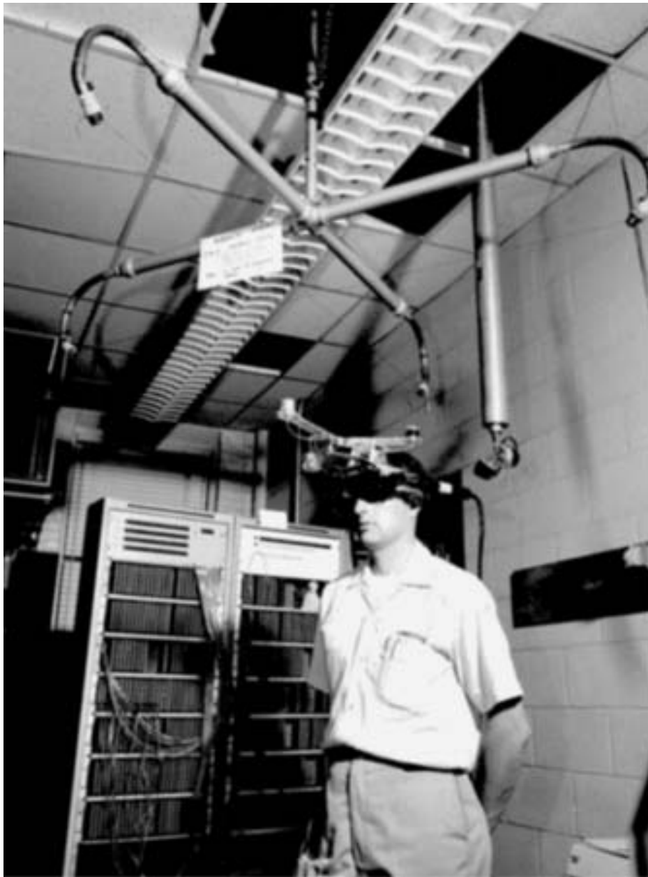
Fig. Early head-mounted display device developed by Ivan Sutherland at Harvard University, c. 1967. Courtesy of Ivan Sutherland
