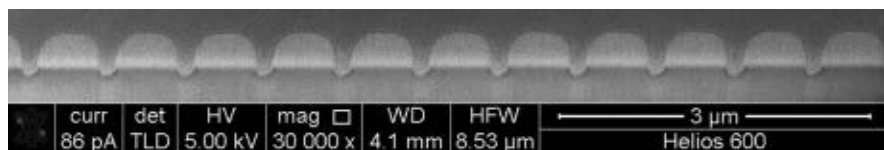
A cross-sectional scanning electron microscopy image of a 750-nm period grating, fabricated by focused ion beam milling in a 300-nm-thick amorphous germanium antimony telluride film on silica.
