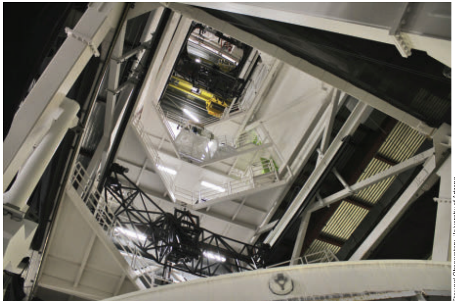
A 28-m-tall testing tower housing a set of four metrology systems that provide independent measurements of the Giant Magellan Telescope segments to guide the computer-controlled optical surfacing process at the Richard F. Caris Mirror Lab, Steward Observatory, University of Arizona.
