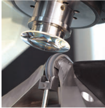
Precision figure correction with magnetorheological finishing, displaying deterministic polishing for superior surface control while providing increased yield.
