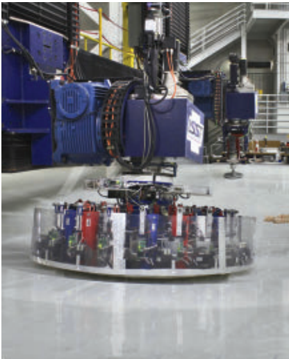
An 8.4-meter mirror for the Large Synoptic Survey Telescope being fabricated using a stressed lap and a non-Newtonian lap at the Richard F. Caris Mirror Lab, Steward Observatory, University of Arizona.
