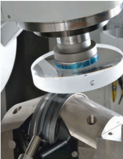
Deterministic polishing of a large aperture lens using magnetorheological finishing.
