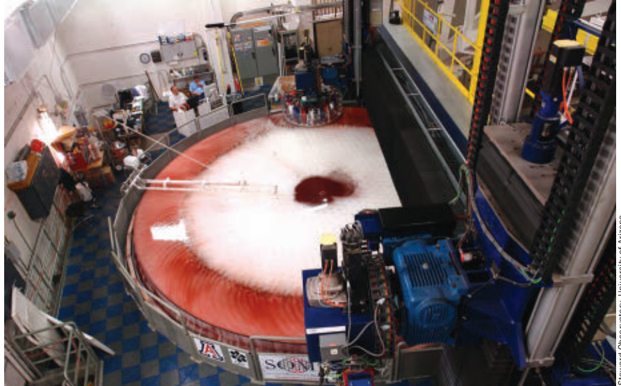
An 8.4-m primary off-axis segment mirror for the Giant Magellan Telescope being fabricated using a stressed lap at the Richard F. Caris Mirror Lab, Steward Observatory, University of Arizona.
