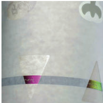
Nanotech Security Corp.'s magenta-to-green color-shift optical thin-film thread shown in unprinted composite banknote material.
