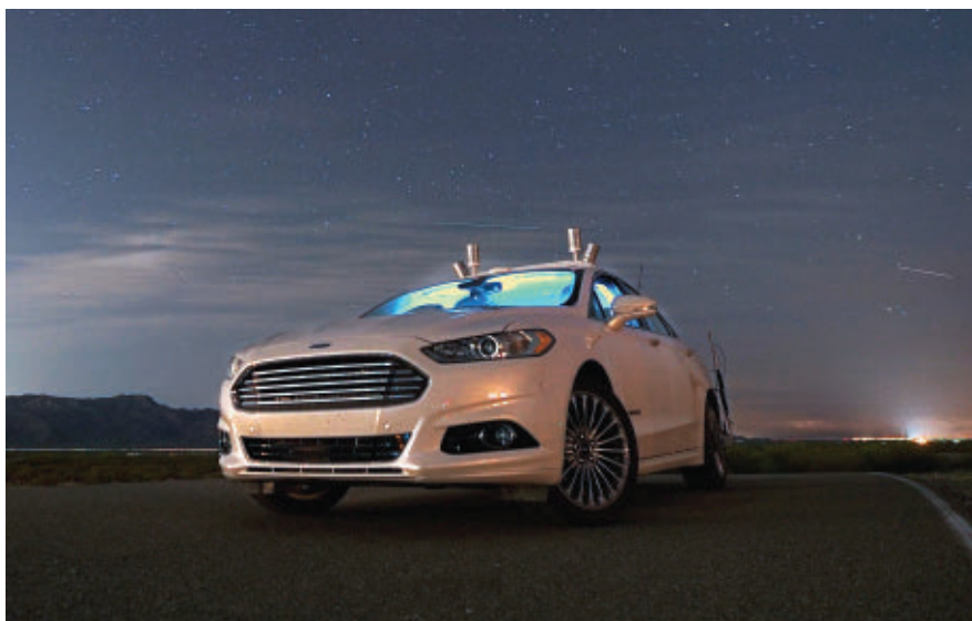
Under the cover of night, a Ford Fusion Hybrid autonomous research vehicle — with no headlights on — navigated along lonely desert roads, performing a task that would be perilous for a human driver.
