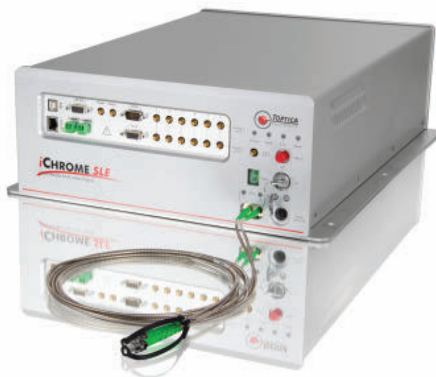
Toptica’s multilaser engine iChrome SLE provides eight laser lines out of one box. It has two output fibers with integrated switch, automated alignment and laser cartridges that enable exchanges in the field.
