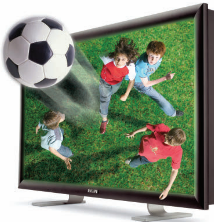
The 42-in. autostereoscopic 3-D display by Philips uses the 2D-plus-Depth format, including Declipse, which gives additional occlusion information for a real 3-D "look around" effect. Courtesy of Philips.
