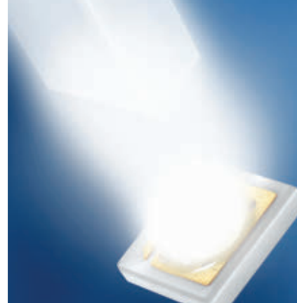
Osram Opto Semiconductor's Oslon LX LEDs, 1-W LEDs for backlighting LED displays, pack almost 80 percent of their light into the lightguide with the aid of an optimized lens, allowing the display to be made ultrathin and uniformly illuminated, even with single-side injection. Courtesy of Osram Opto Semiconductor.
