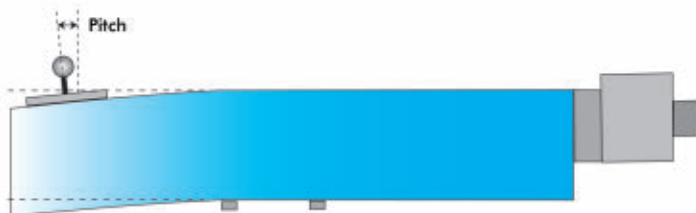
Figure 2. If a stage is not fully supported, pitch errors can occur when a load moves toward the unsupported side of the stage.
