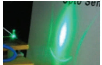
Direct green InGaN-based laser emission with CW output of 50 mW is a milestone for mobile laser projection technology. Courtesy of Osram Opto Semiconductors.
