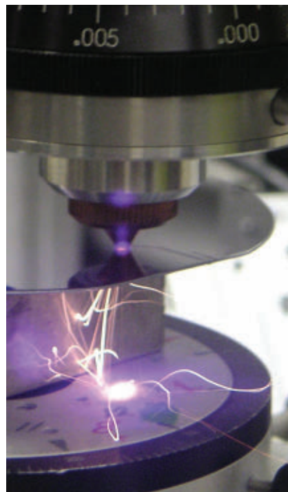
A fiber laser cuts silicon. Courtesy of SPI Lasers.
