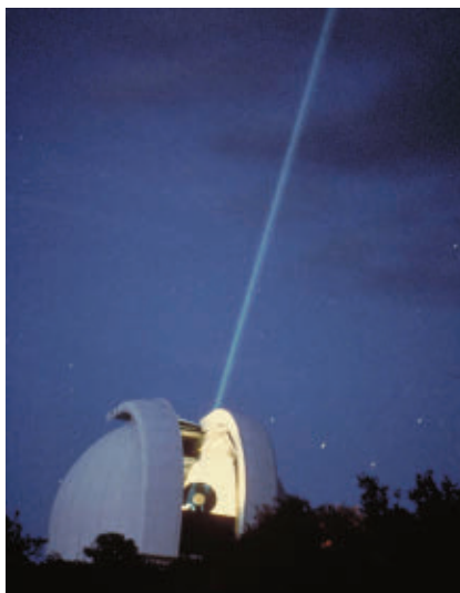
For almost 20 years from the late 1960s, astronomers measured the Earth-to-moon distance by beaming a laser from the 2.7-m McDonald Observatory Smith Telescope to retroreflectors placed on the moon. Courtesy of McDonald Observatory.
