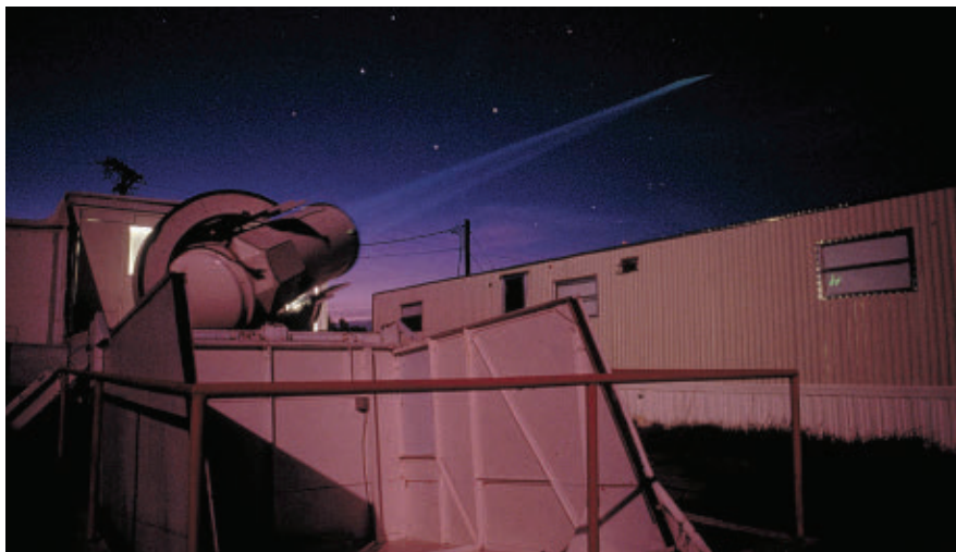
Earth-moon measurements are now preformed with a dedicated telescope, the McDonald Laser Ranging Station. Photo by Kathryn Gessas, McDonald Observatory.
