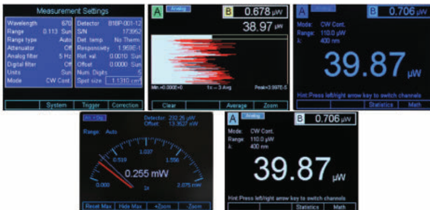
Figure 3. Advanced optical power meters feature a number of graphical display options.
