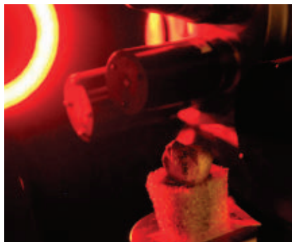
Several of Lucy's skeletal elements, including the right distal radius (arm bone), were scanned with an ultrahigh-resolution Xradia MicroXCT scanner in the High-Resolution X-ray CT Facility at the University of Texas at Austin. Custom-built foam mounts were constructed to safely hold the specimens in the scanner. Photo by Marsha Miller, courtesy of University of Texas at Austin.
