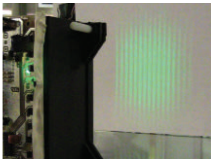
A high-speed solid-state projector labels space by emitting near-infrared patterns of light at 870 nm. Imperceptible photosensors hidden underneath a subject's clothes receive a distinct pattern from the sequence and, by doing so, determine their own location. The projectors encase an LED and passive binary film that transmit the patterns of light.
