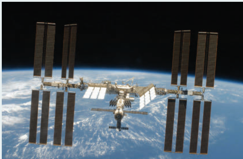
The International Space Station is powered by four solar arrays that produce about 120 kW of electricity. Courtesy of Boeing Corp.
