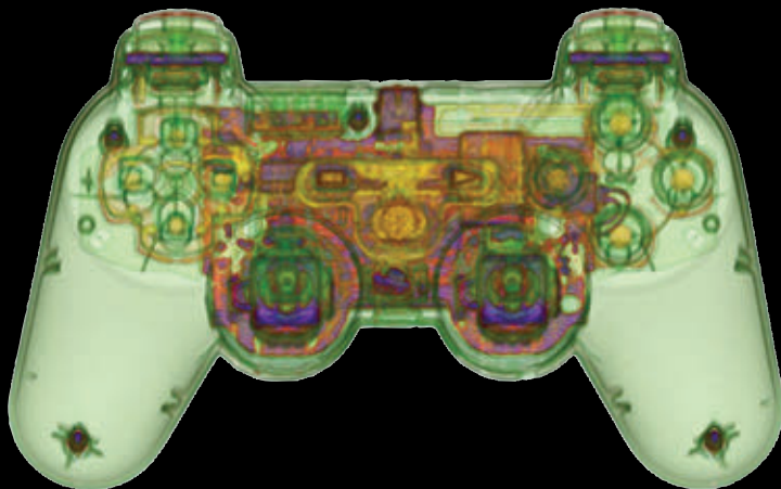
Above, the detailed electronic mechanism of a wireless remote from a Playstation 3 game system is shown in this scan. The circuit board can be seen, as well as the surface knobs and buttons.
