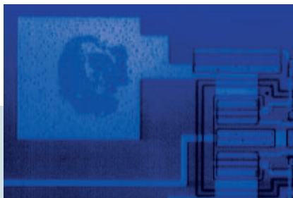
Near-IR inspection can detect details and defects not visible otherwise, particularly since silicon is transparent to near-IR. The image on the right is from a standard microscope equipped with near-IR, while the one on the left is from a high-resolution laser confocal microscope. Courtesy of Olympus America.
