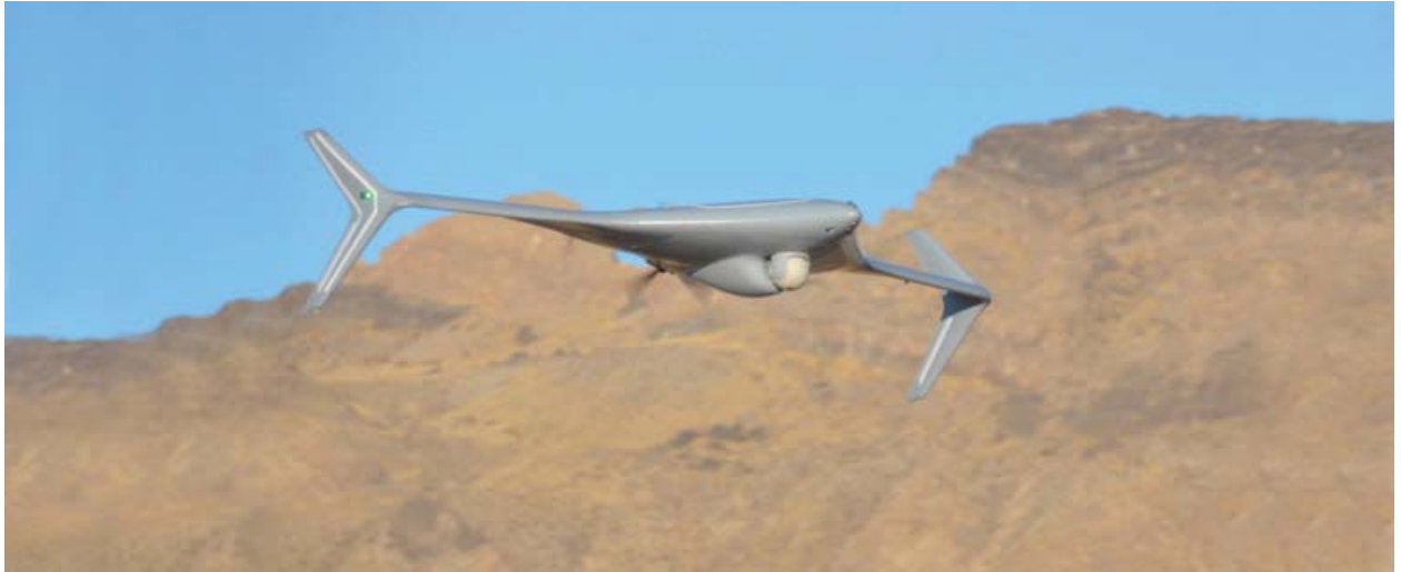
3. The Bat series of UAS devices are constructed with large wingspans to handle multiple EW sensor payloads. (Courtesy of Lockheed Martin Corp.)
