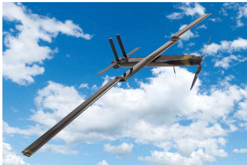
2. The Outrider, a compact UAS, can be launched from canisters that fit inside submarine missile tubes. (Courtesy of Lockheed Martin Corp.)
