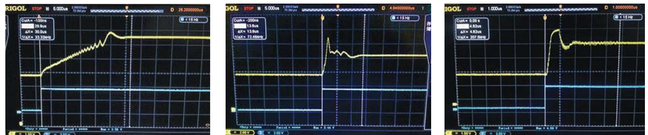
6. The oscilloscope screenshots show the lock times for the PLL synthesizers, with (left) a 150-kHz static loop bandwidth, (middle) a model ADF4154 as the PFD, and (right) a model ADF4193 as the PFD.
