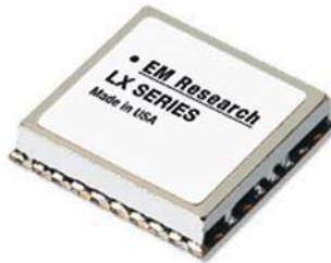
2. The compact LX series of phase-locked frequency sources includes this 840-MHz unit with low phase noise. (Photo courtesy of EM Research, www.emresearch.com )
