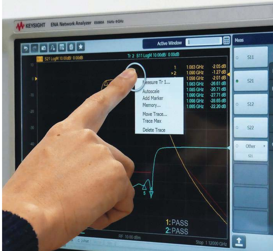
2. The E5080A ENA analyzers feature a 12.1-in. TFT LCD touchscreen display that allows multiple highlight zones.
