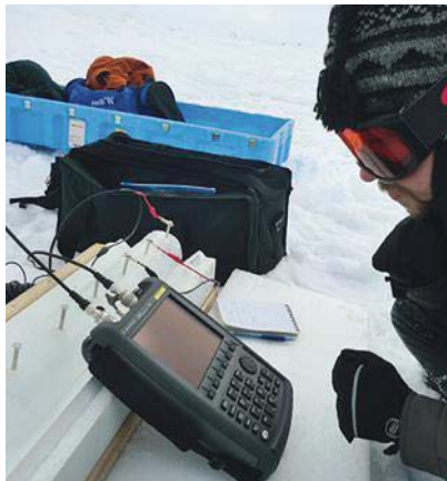
8. The portable FieldFox analyzer, which readily makes measurements to 26.5 GHz in the field, represents just one of the many instruments on display at the upcoming 2015 IMS Exhibition in Phoenix, Ariz. (Photo courtesy of Keysight Technologies, www.keysight.com )
