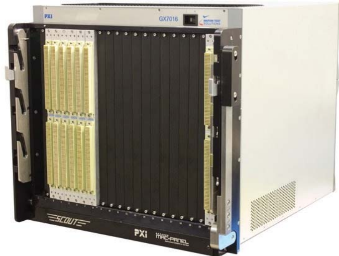
2. An important part of the TS-323 GENASYS system is the GX7016 switching receiver subsystem, housed in a 20-slot 6U PXI chassis.
