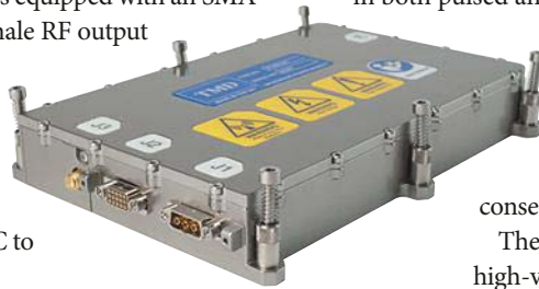
2. The PTXM series of TWTAs includes broadband, compact models capable of more than 100 W output power across wide bandwidths to 18 GHz.
