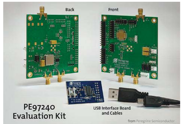
3. This evaluation board was developed to support the model PE97240 PLL synthesizer for applications to 5 GHz. (Photo courtesy of Peregrine Semiconductor Corp., www.psemi.com .)
