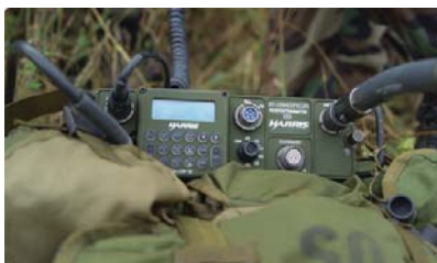
1. The FALCON II AN/PRC-150(C) manpack radio system employs SDR technology to achieve excellent signal security. [Photo courtesy of Harris Corp. ( www.harris.com )]
