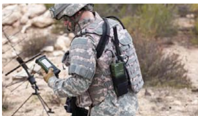
2. The Falcon III AN/PRC-152 single-channel multiband radio provides secure communications from 30 to 512 MHz. [Photo courtesy of Harris Corp. ( www.harris.com )]
