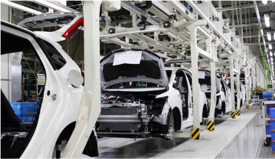
By introducing cutting-edge production technology, the Honda Yorii Plant has achieved a tact time of less than 50 seconds for the production of the FIT.
