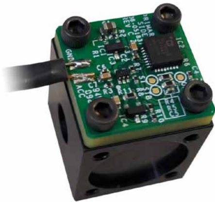
Vibration measurement test setup: the EVAL-CN0532-EBZ board attached to a shaker table using an aluminium mounting block.
