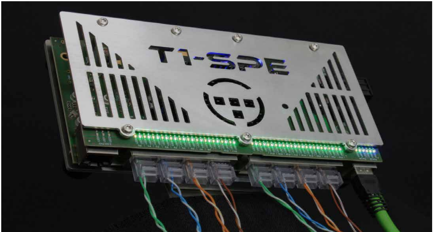
Single Pair Ethernet Evaluation Board with RJ45 jacks.
