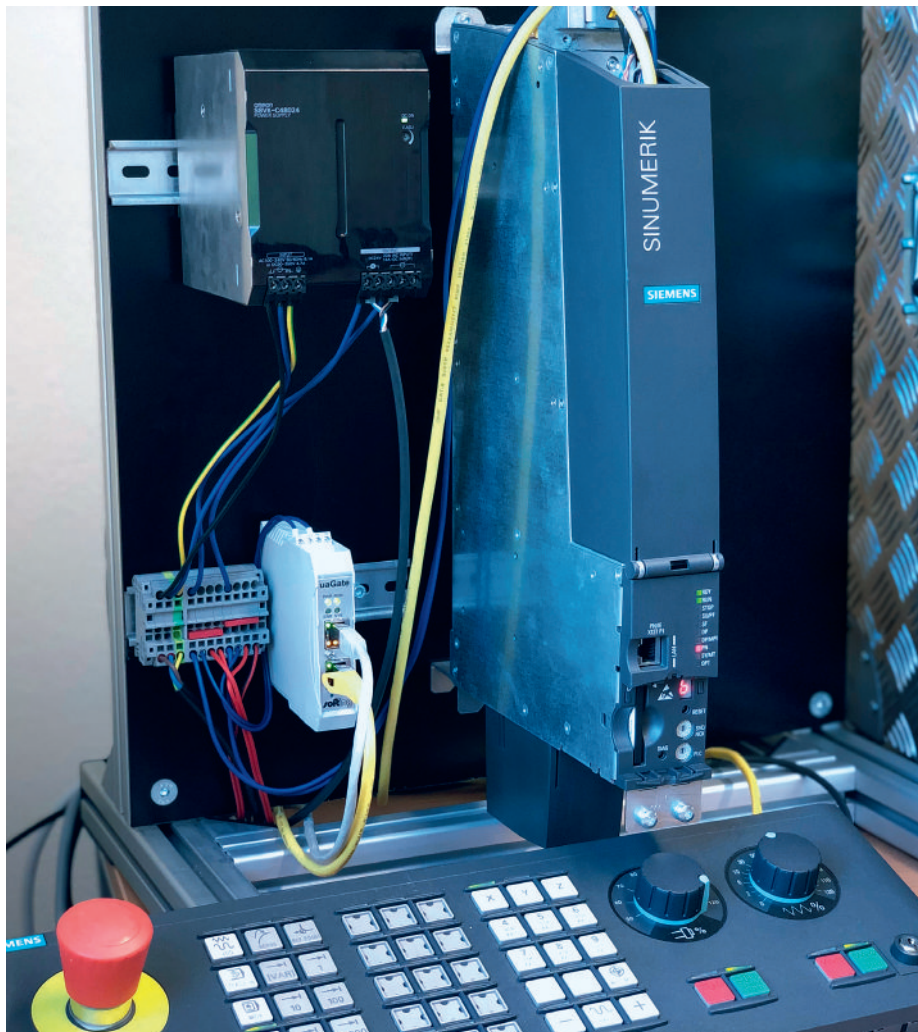
The uaGate 840D gateway can be connected directly to the SINUMERIK 840D pl CNC controller without requiring a system adaptation and any additional licenses.
