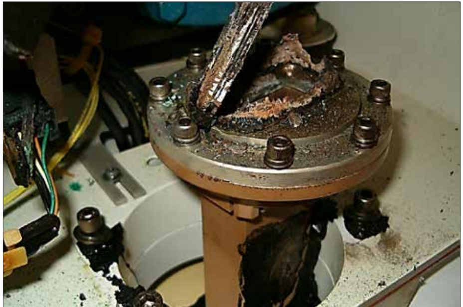
Figure 7 • Moisture ingress can cause device failure by changing the electrical characteristics and increasing the power dissipating in a connection, such as a rotary connector. Source: http://www.microwaves101.com/mortuary/993-microwave-mortuary-2011 .
